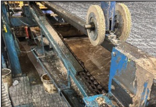
The chain conveyor transporting carpet from the tufting machine.
